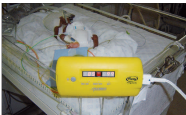
The wind-up pulse oximeter being used to measure the oxygen saturation of a preterm infant with respiratory distress receiving continuous positive airway pressure support.
