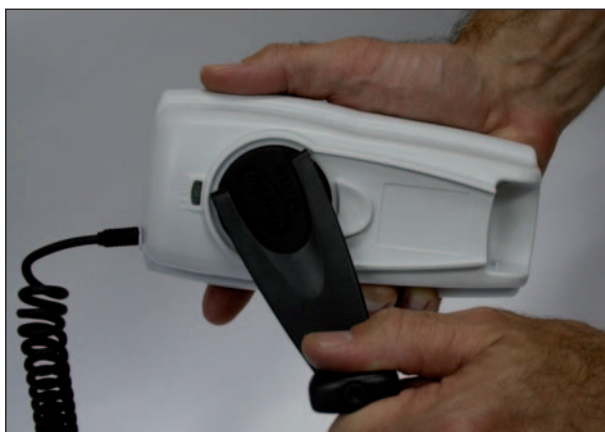
Demonstrating the hand crank to recharge the batteries of the Doppler ultrasound fetal heart rate monitor. One minute of winding provides 10 minutes of monitoring.
