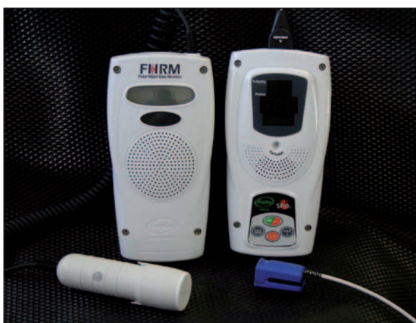
The wind-up fetal heart rate monitor together with a wind-up pulse oximeter. Both would improve the emergency care of women in labour.
